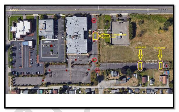
Structures requiring service circled in red for catch basins and pink for Contech. 3 of 13 catch basins need service. 2 of 2 Contech cartridge bays need service. Cartridge vault needs cleaning and Contech cartridge replaqcement
